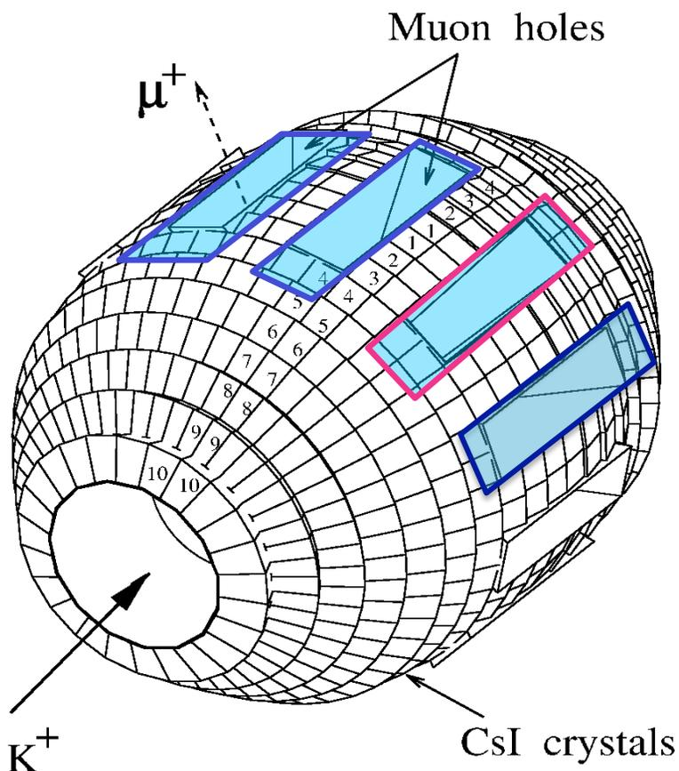
**12 C1 triple-GEMs** to cover muon gaps of CsI(Tl)
