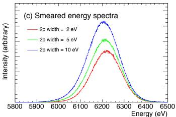
Nd-filtered spectra measured with SDD width 2, 5, 10 eV
