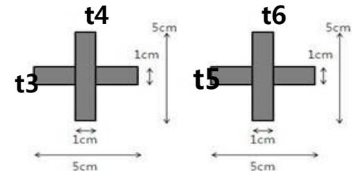
**Beam Trigger:  $t3 \otimes t4 \otimes t5 \otimes t6$**
